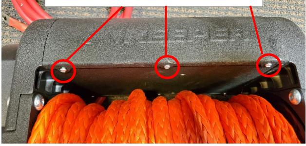
For **KX9500E**, **KX9500ES** and **KX9500EH** Winches Remove top cover by removing 4 Philip screws. There are 2 screws in the front top and 2 screws in the back top.
